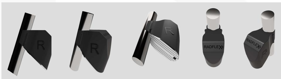
RADFLEX® BRR is Designed for the most common seat post's with diameter 22-32mm as well as for aerodynamic seat post's. Aerodynamic shaped in plastic weighs only 35gram and have small size 65 x 80 x 40mm, the construction includes built in "snap on" for the seat post equipped with bracket's for a strap (included).
